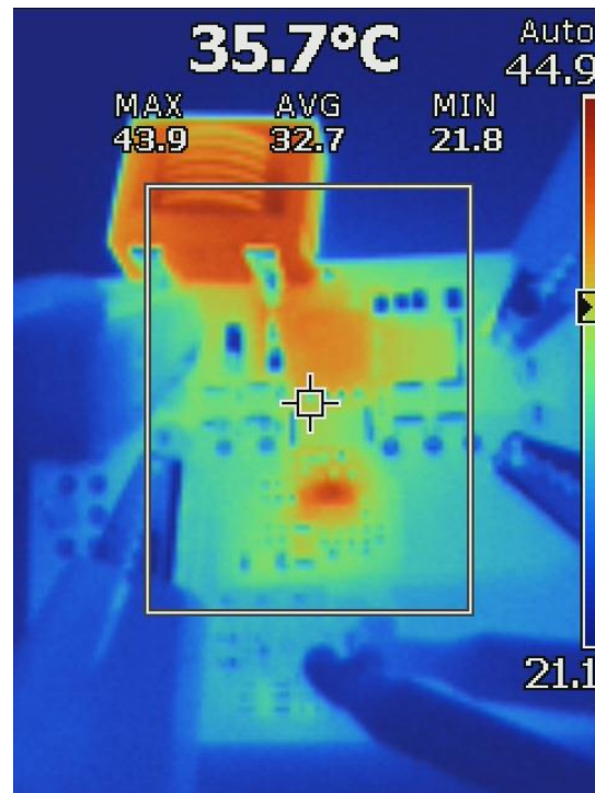
Figure 6. Thermal Image, 24V Input, 40-V Output at 100 mA Load
