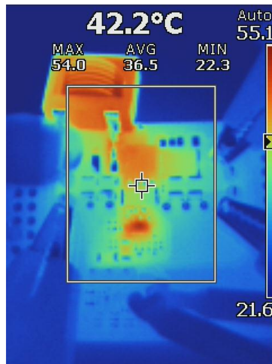
Figure 7. Thermal Image, 24V Input, 60-V Output at 100 mA Load
