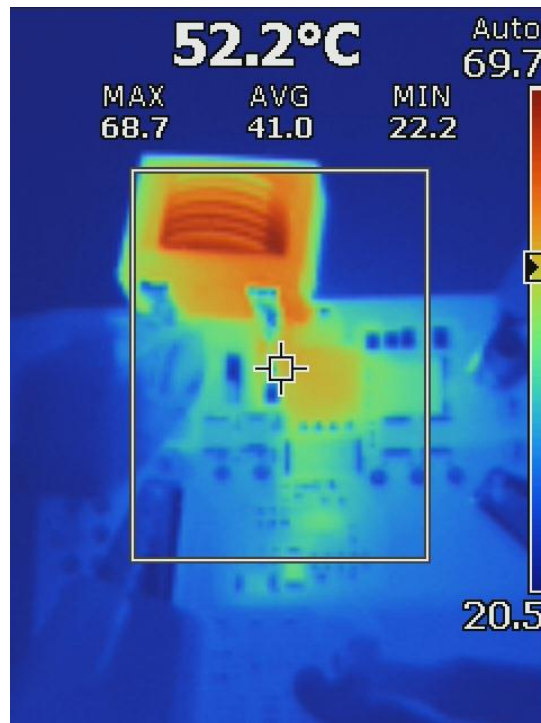
Figure 5. Thermal Image, 6-V Input, 80-V Output at 100 mA Load
