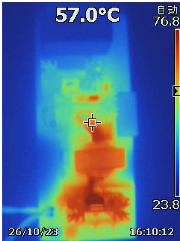
Figure 2-10. Thermal Image 1000 V IN 12 V, 4-A Load Top View
