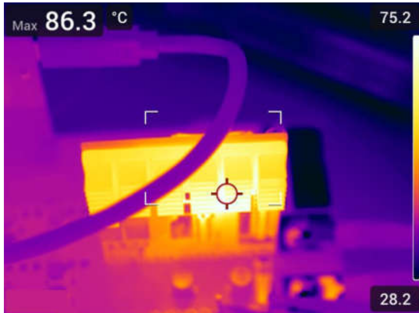
Figure 3-4. Thermal Image at 28.6V V_{in} , 50V V_{out} , and 22A I_{out}
