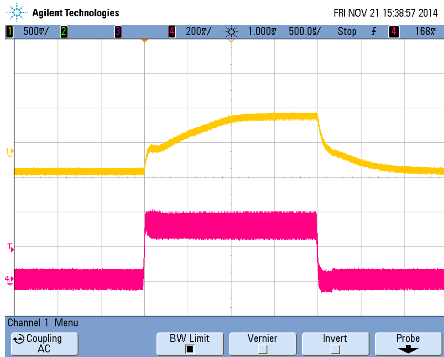
Figure 17 VEE_B output load transient
