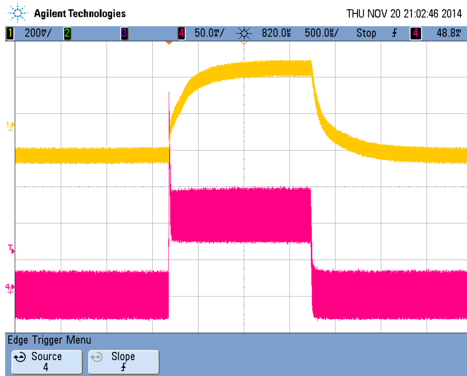
Figure 19 VEE_U_T output load transient
