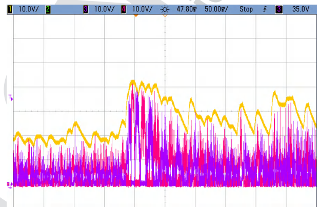
Figure 3-2. Audio Output and Boost Voltage With Class-H Operation
