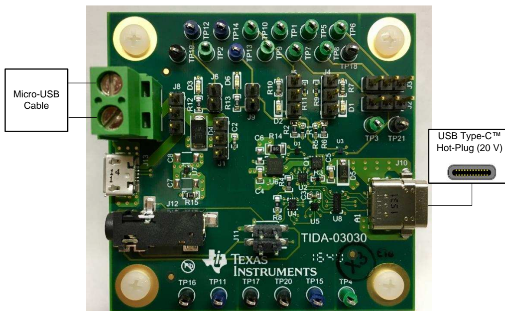
Figure 6. Power Path Protection Test Setup
