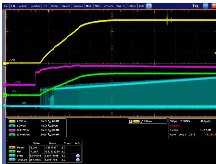
Figure 3. 阻性负载起机波形 Ch1=Vout, Ch2=SW, Ch3=Comp, Ch4=inductor current
