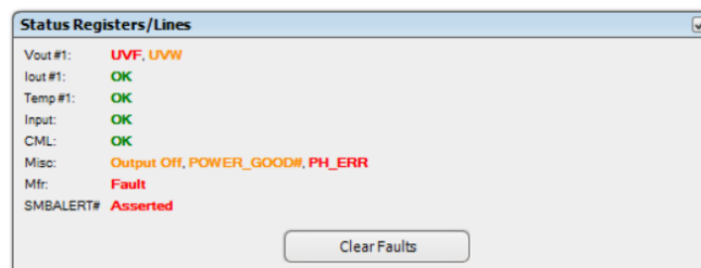
Figure 7. OCL 故障记录
