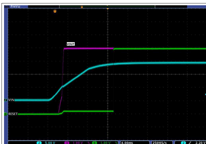
Figure 23. TPS7B6750-Q1 Power-Up Waveform
