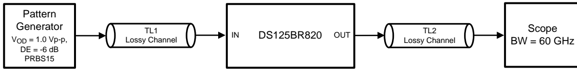
Figure 10. Test Setup Connections Diagram
