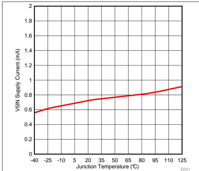
Figure 1. V5IN Supply Current vs Junction Temperature
