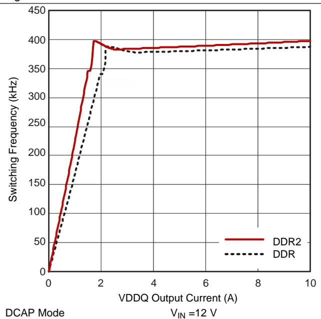
Figure 10. Switching Frequency vs I<sub>VDDQ</sub> Output Current
