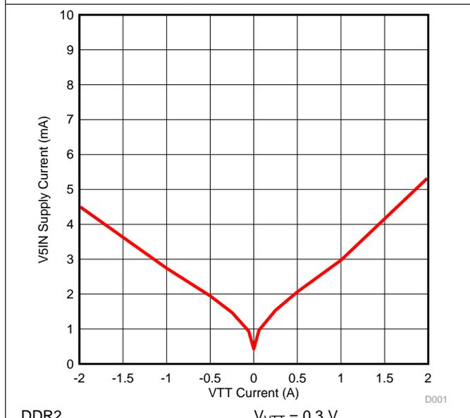
Figure 3. V5IN Supply Current vs VTT Current
