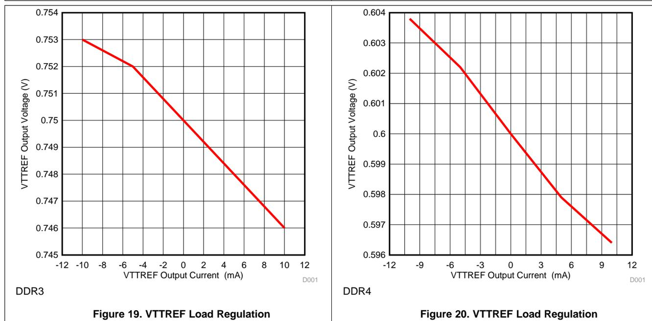
Figure 19. VTTREF Load Regulation
