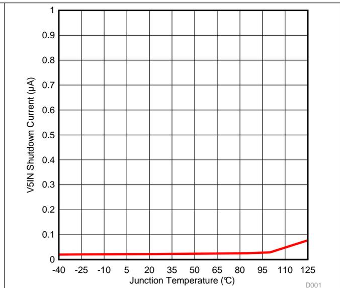
Figure 2. V5IN Shutdown Current vs Junction Temperature
