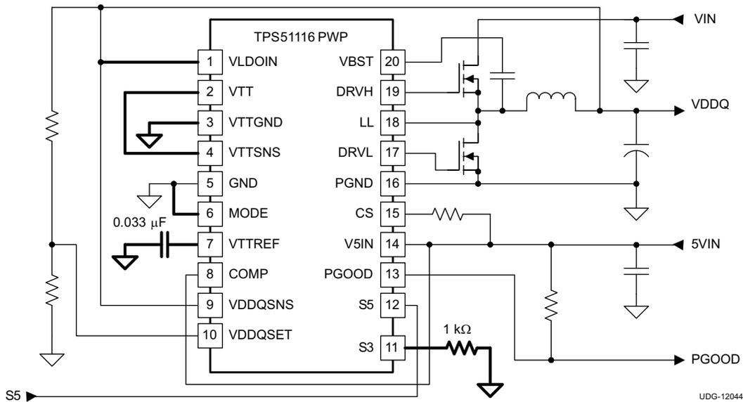
Figure 34. Application Circuit When VTT Is Not Required
