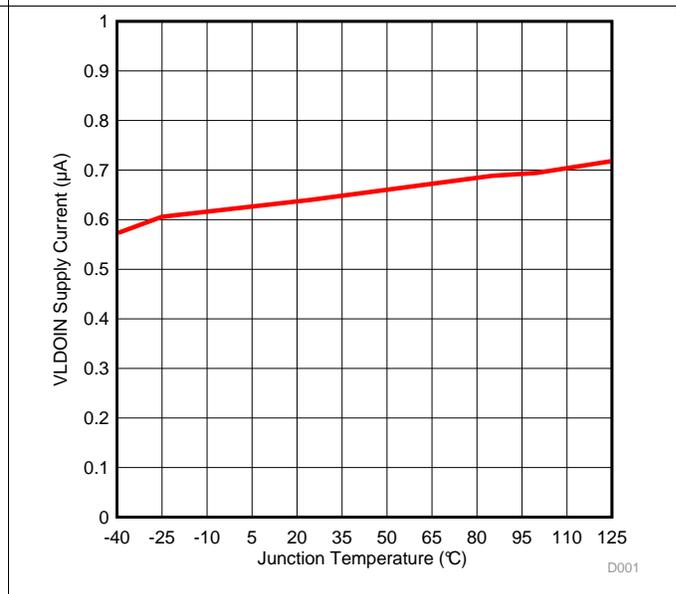
Figure 4. VLDOIN Supply Current vs Junction Temperature
