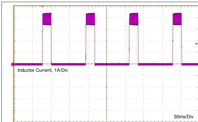
图 8-5. Inductor Current Burst in Short-Circuit Mode
