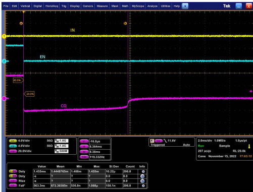
图 9-4. OUT In Current Fault Auto Recovery, Low Side Mode
