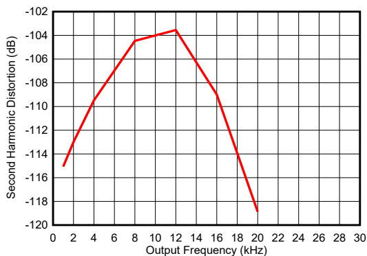
DAC update rate = 768 kHz, V_{REFPF} = 4.5\text{ V} , V_{REFNF} = -4.5\text{ V} , sixth-order, low-pass, 30-kHz output filter
