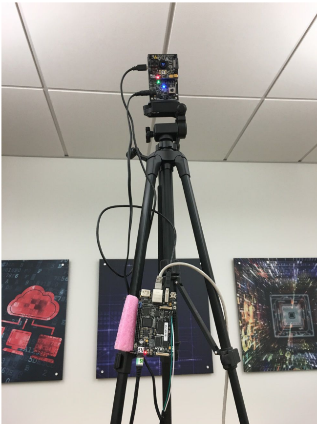
图 26. OPT8241 CDK and Rico Board on Tripod
