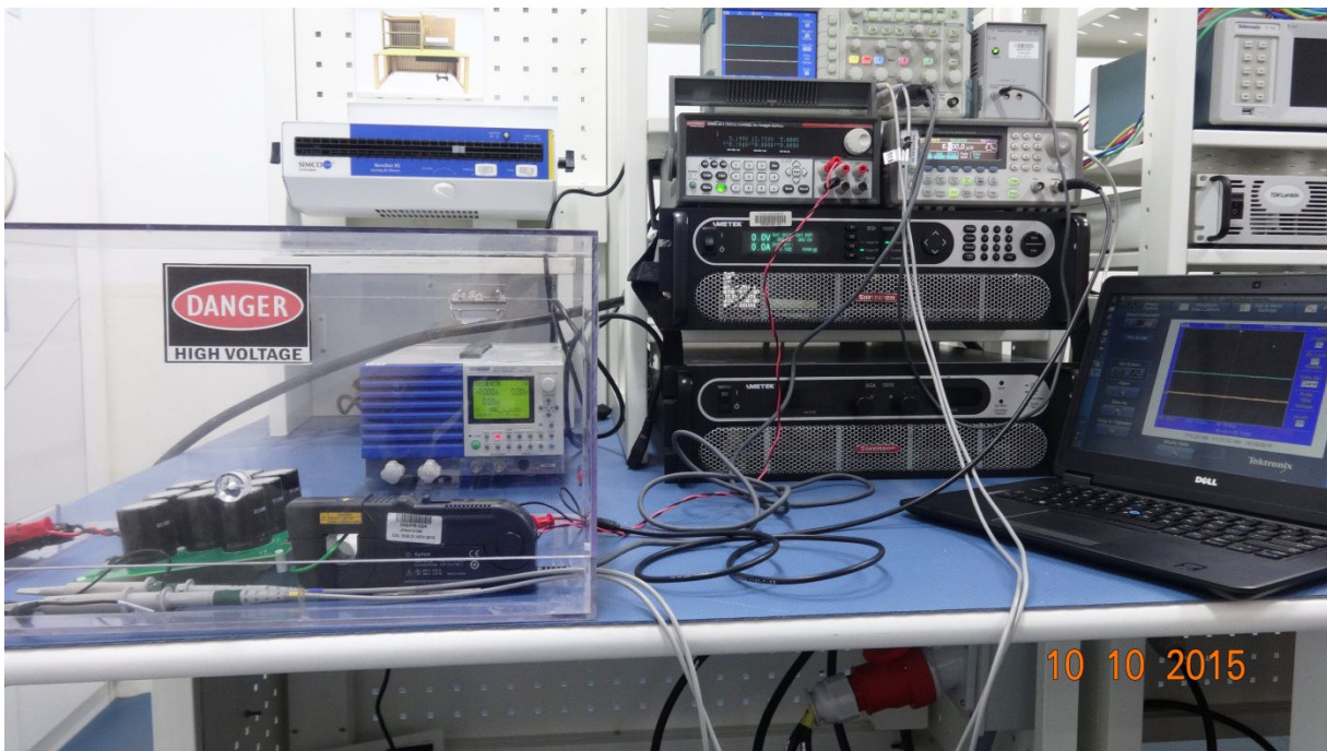
图 75. Miller Clamp and Desaturation Detection Test Setup
