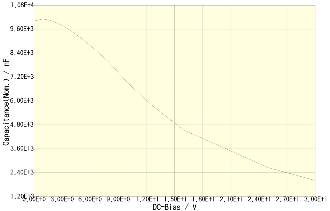
图 7. Variation of Capacitance With Applied DC Bias for C3216X7R1V106K160AC
