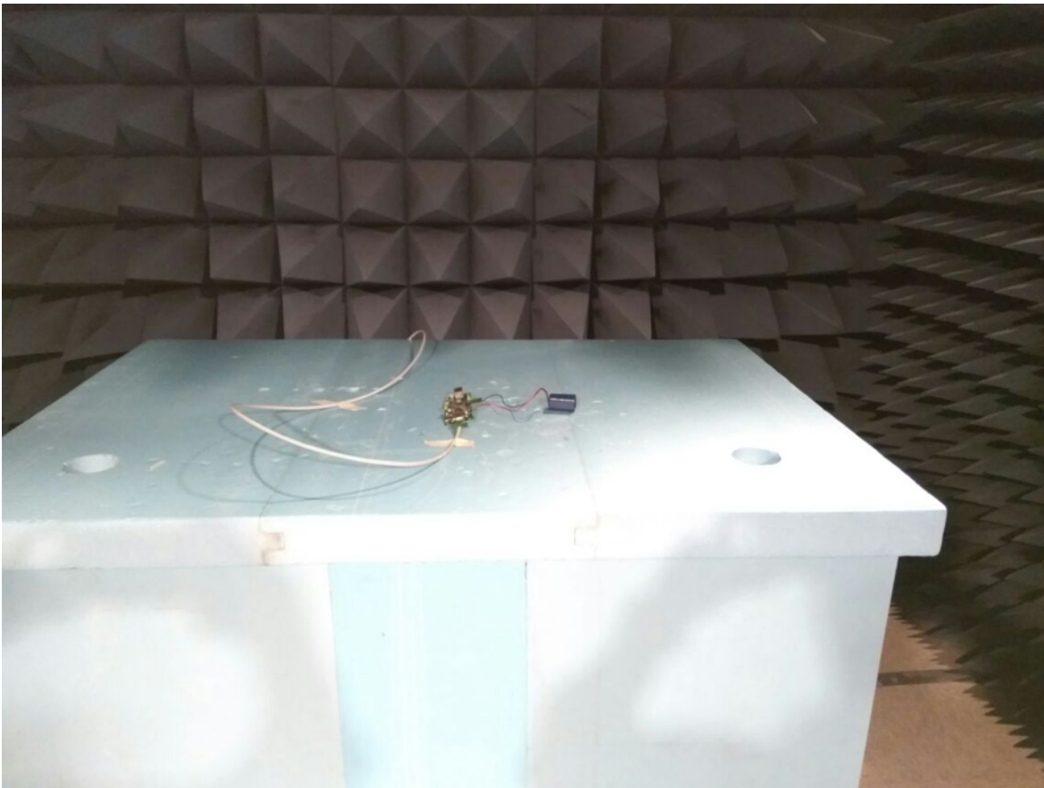
图 25. Ethernet PHY + Controller During Radiated Emission Test
