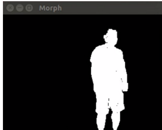
图 11. Morphology Filter on Binary Image
