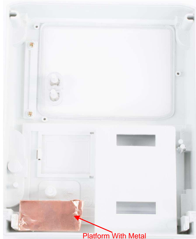
图 25. Case Platform With Metal Placed on Top
