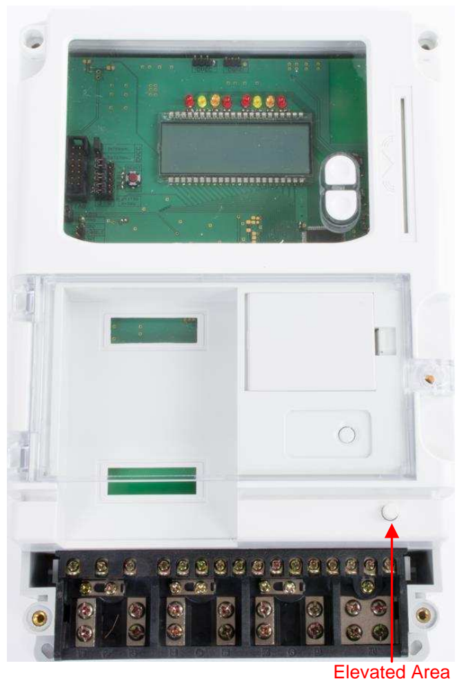
图 23. Main Cover Placed on e-Meter Case
