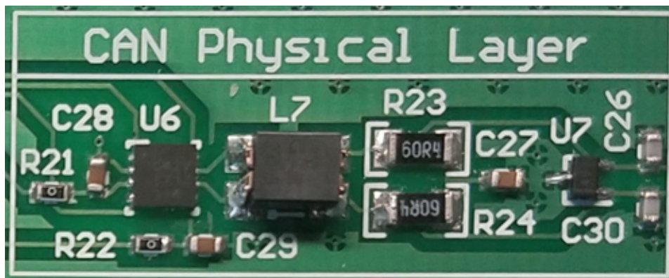
图 14. CAN Physical Layer Circuitry on PCB
