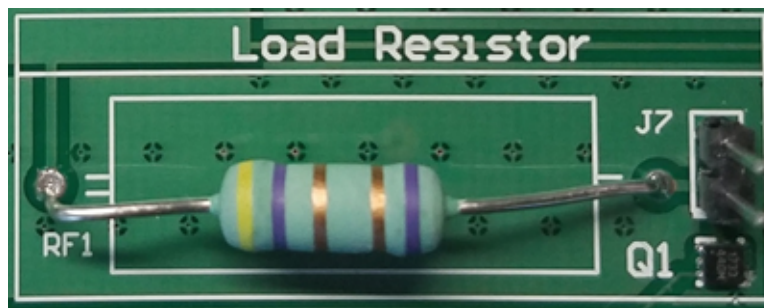
图 18. Dummy Load Resistor Circuitry on PCB
