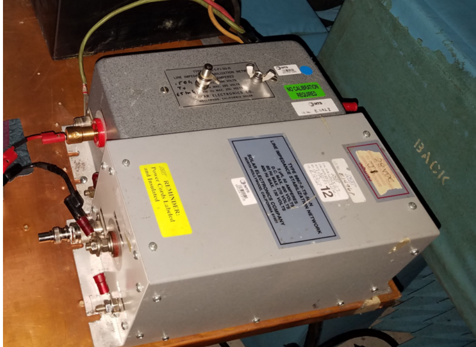
图 50. Two Artificial Networks With Measuring Ports for Conducted Emissions Testing
