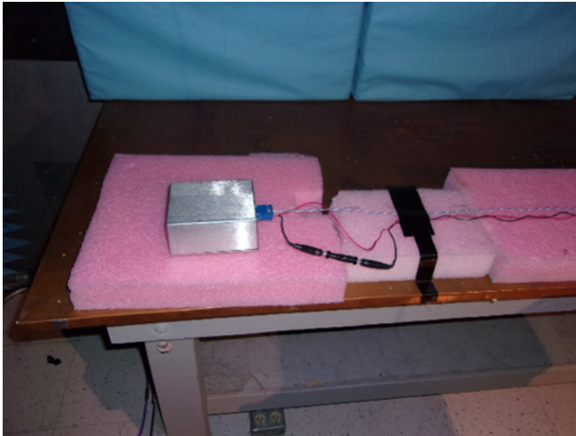
图 37. Slave Node Setup for RE per CISPR 25 ALSE
