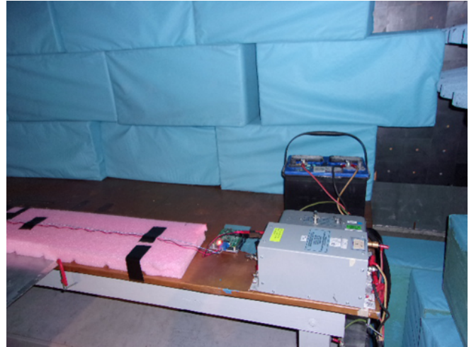
图 52. Master Node Setup for Radiated Emission
