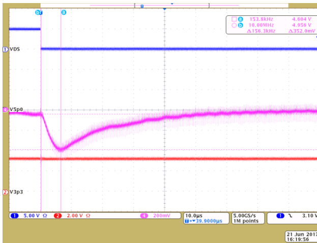
图 45. Buck Converter Load Step Increase Response
