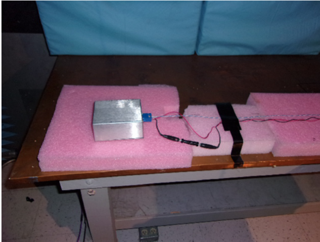
图 51. Slave Node Setup for Radiated Emissions
