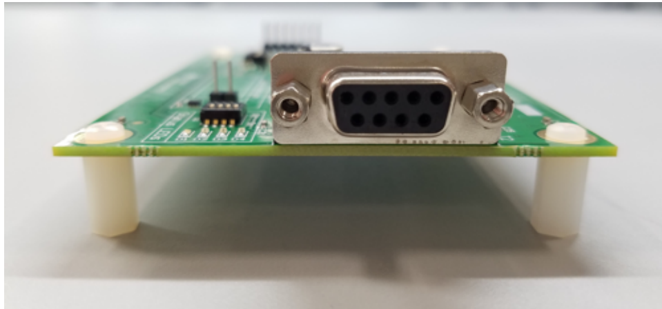
图 21. External Connector for Power and CAN on PCB
