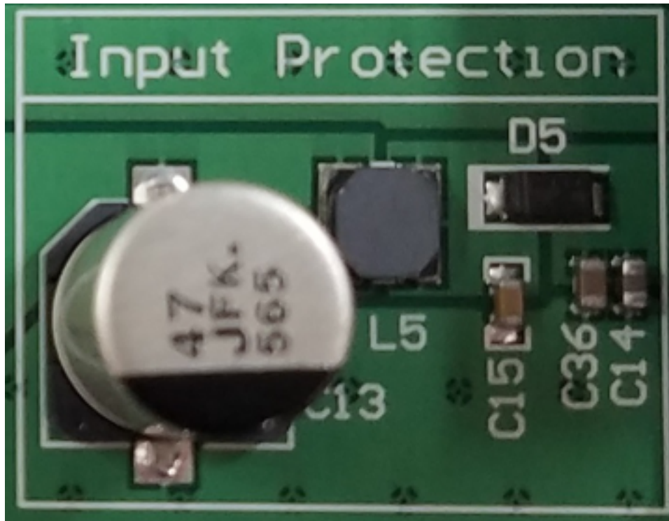
图 11. Battery Filtering and Protection PCB Snippet
