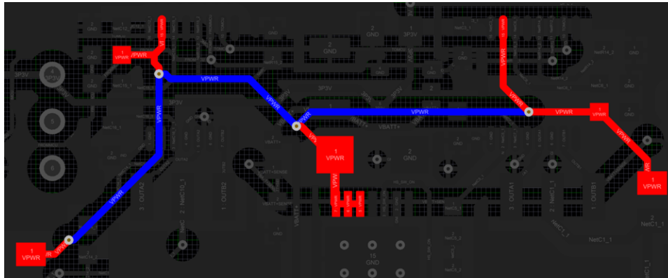
图 69. Routing of VPWR Routing From High-Side Switch to PGA460-Q1 Devices and Transformers
