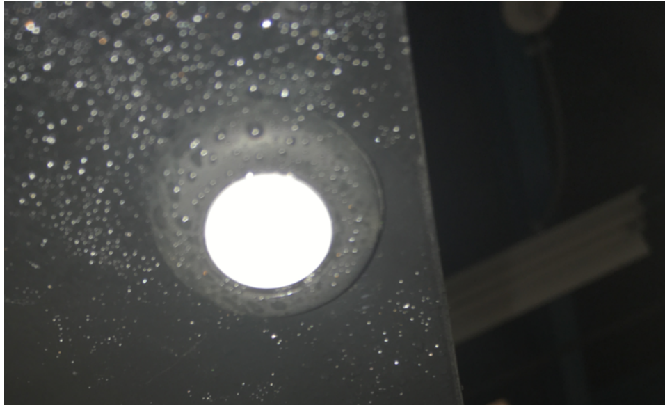
图 54. Water Applied to Bumper Cover and Ultrasonic Sensor
