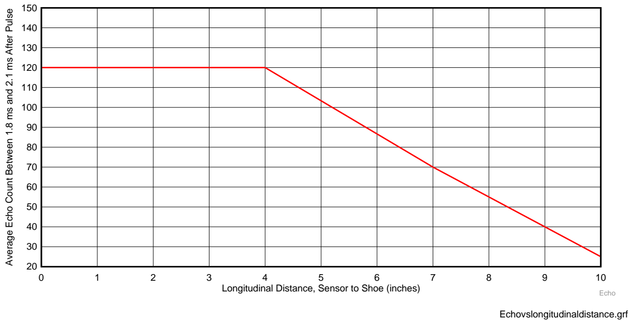
图 53. Effect of Kicking Gesture Directed at Point Displaced From Ultrasonic Transducer
