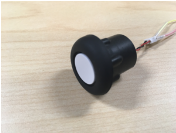
图 11. Closed-Top Murata Ultrasonic Transducer in Rubber Mounting Sleeve
