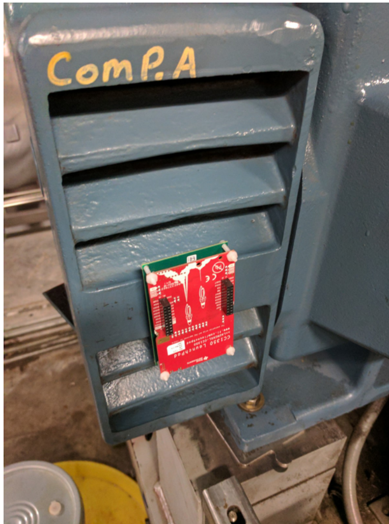
图 14. Reference Design Coupled to Motor
