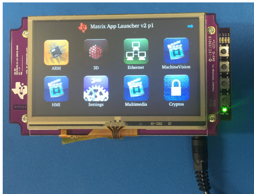
图 5. AM335x Starter Kit Setup (LCD Face Up)
