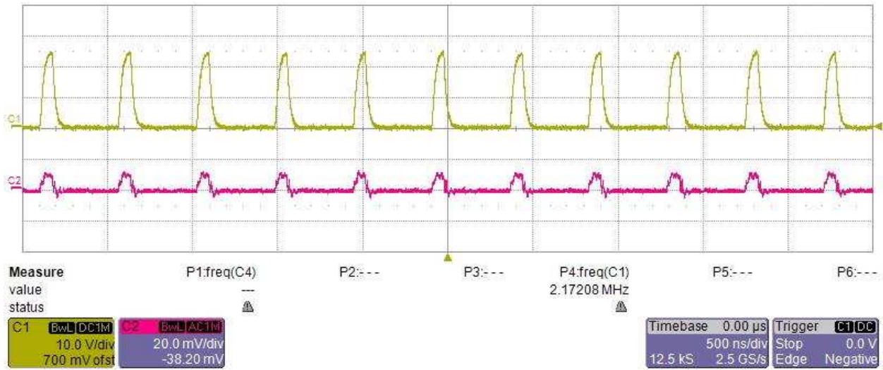
图 21. LM73605-Q1 Switch Node and Output Voltage Ripple, 20-V Input at Full Load
