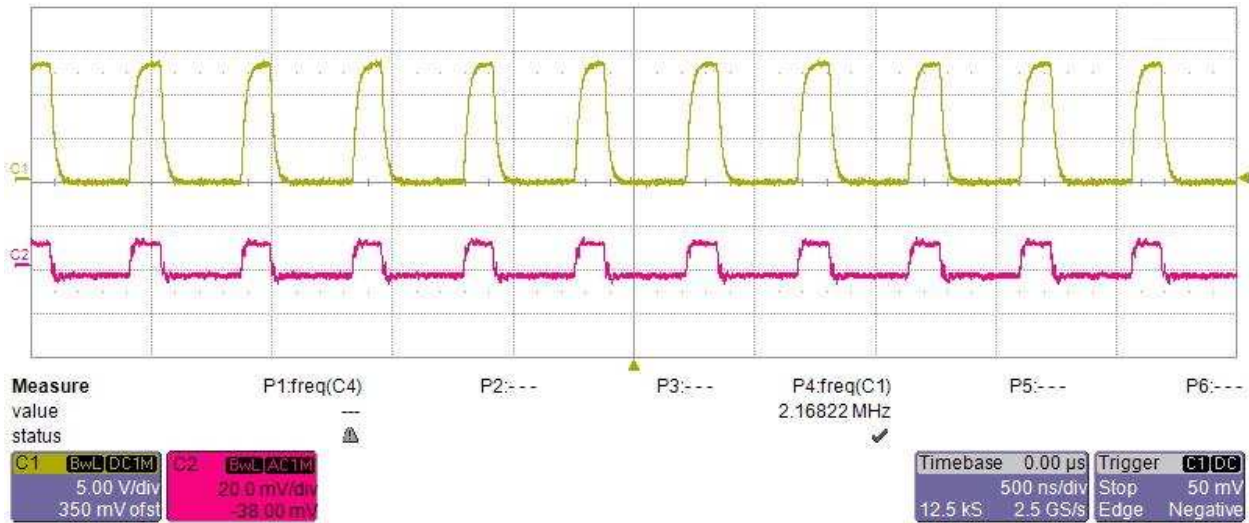
图 19. LM73605-Q1 Switch Node and Output Voltage Ripple, 13.5-V Input at Full Load
