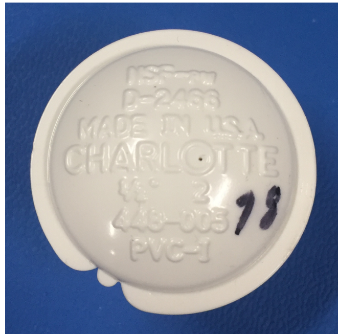
图 5. Cap With Hole for Test Leak Apparatus
