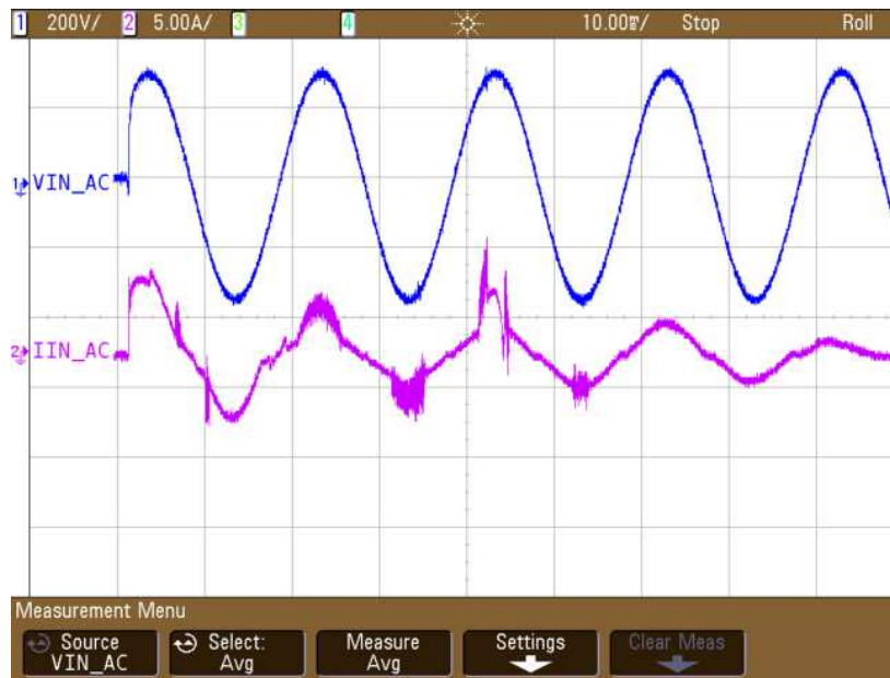
图 7. Inrush Current Limiting at Start-Up
