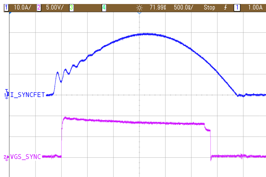
图 14. Synchronous Rectifier Working Waveform
