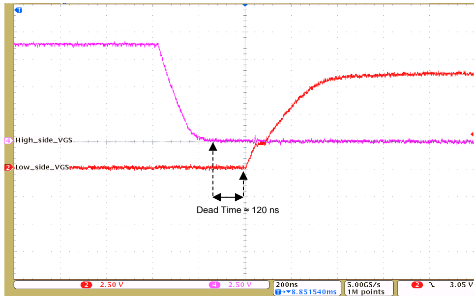
图 16. Dead Time at Rising Edge of Low-Side V_{GS}
