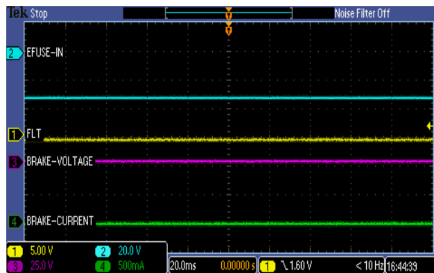
图 21. Reverse-Input Polarity Protection at -30 V
