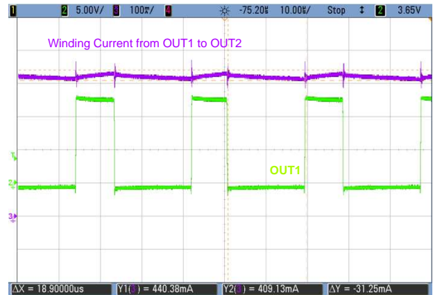
图 28. Current Regulation With Slow Decay Mode
