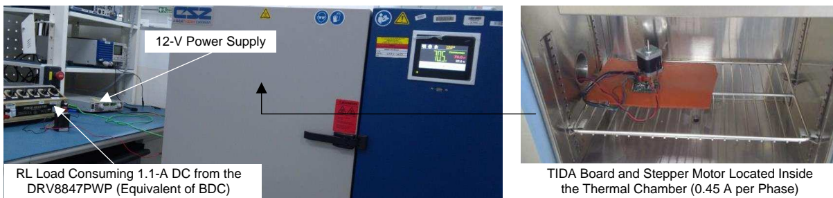
图 45. Setup for Testing the Design at Multiple Ambient Temperatures
