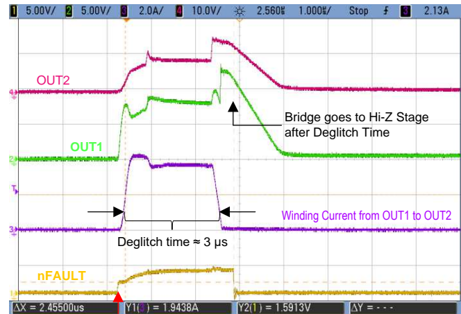
图 37. Short-Circuit Deglitch Time for Noise Tolerant Short Circuit Detection
