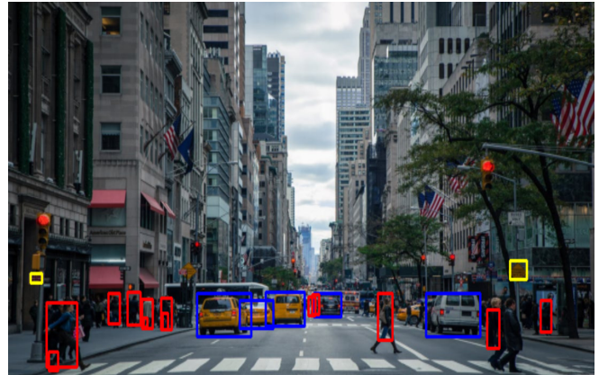
图 18. "ssd_multibox" Output With Detected Objects of Various Classes
