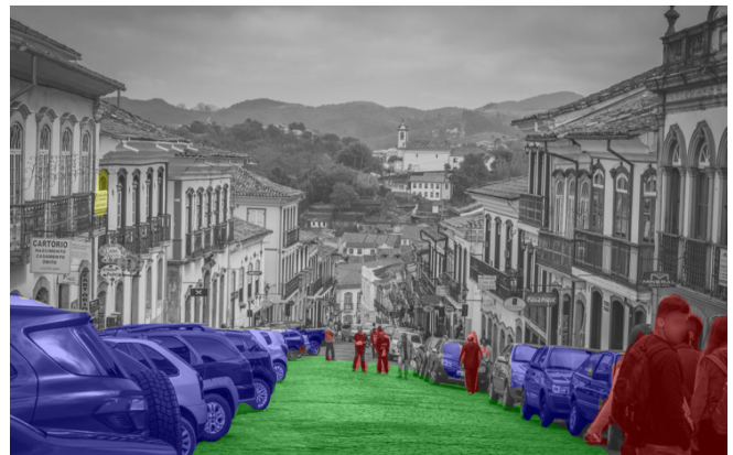
图 20. "segmentation" Output With Pixel Level Classification
