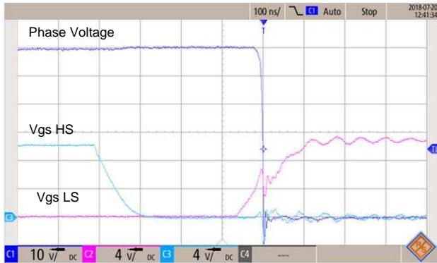
图 14. Hard Switching Phase A Voltage Falling Edge, Phase Current at 60 V, 10 A
