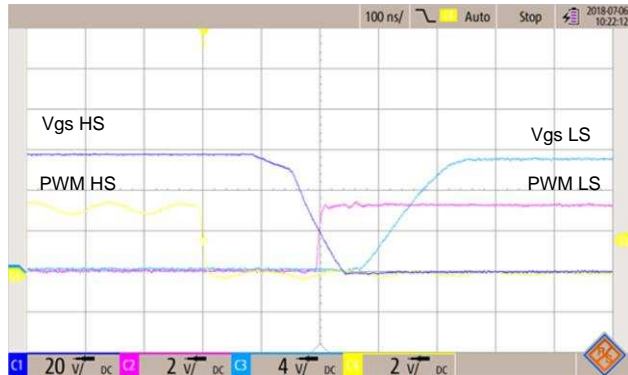
图 24. Independent Mode PWM vs V_{GS} LS and HS, Phase A Current at 48 V, -5 A Soft Switching
