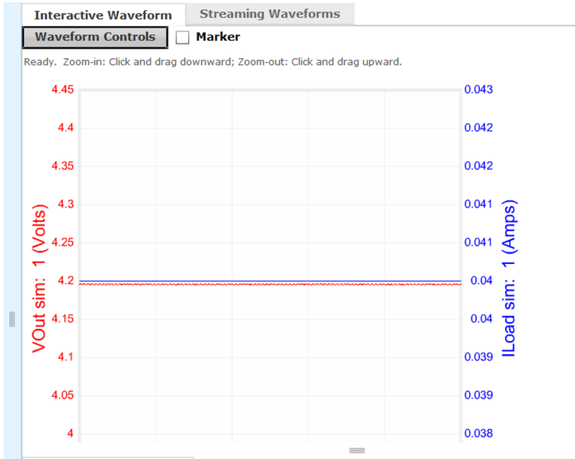
图 11. WEBENCH® Simulation for TPS61099 Boost Converter (Test Results)
