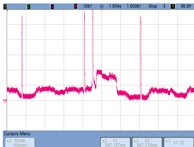
图 48. Pulse Showing Standard BLE Once Connected
