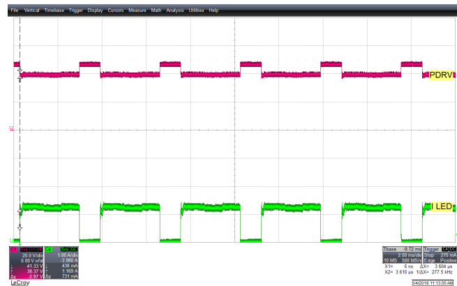
图 12. 240 Hz, 33% Duty Cycle PWM Dimming Feature with R18 (100 K \Omega )—CH1: PDRV, and CH4: LED Current
