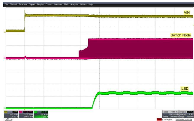
图 10. High Beam/Low Beam Mode Steady State Switching—CH2: Switch Node (Q3 Drain) Voltage and CH4: LED Current for Ouput power of 55 W
