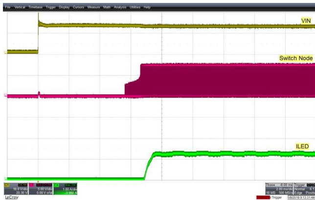
图 9. Low Beam Mode Startup—CH1: VIN, CH2: Switch Node (Q3 Drain) Voltage, and CH4: LED Current
