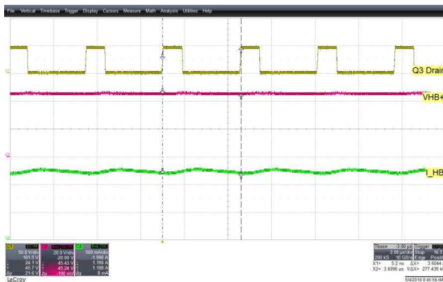
图 11. Normal Operation Fswitch at 275 KHz—CH1: Switch Node (Q3 Drain), CH2: VLED in High Beam and Low Beam Mode, and CH4: LED Current for Ouput power of 55 W
