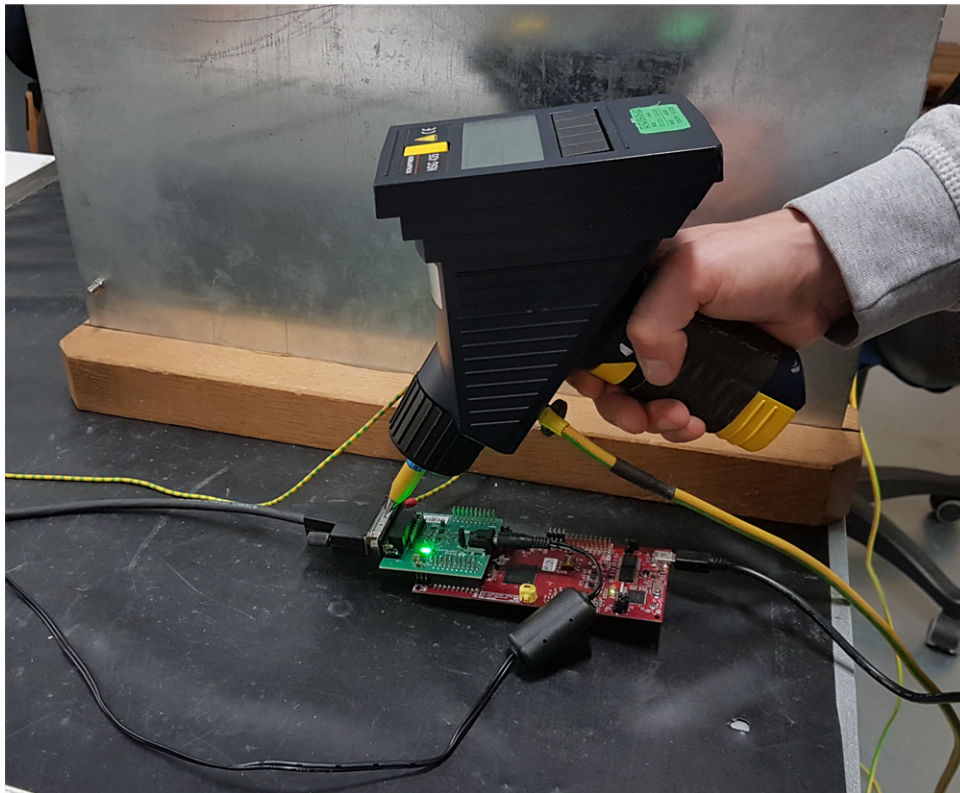
图 48. TIDA-010026 Test Setup for ESD Immunity Tests Using Encoder
