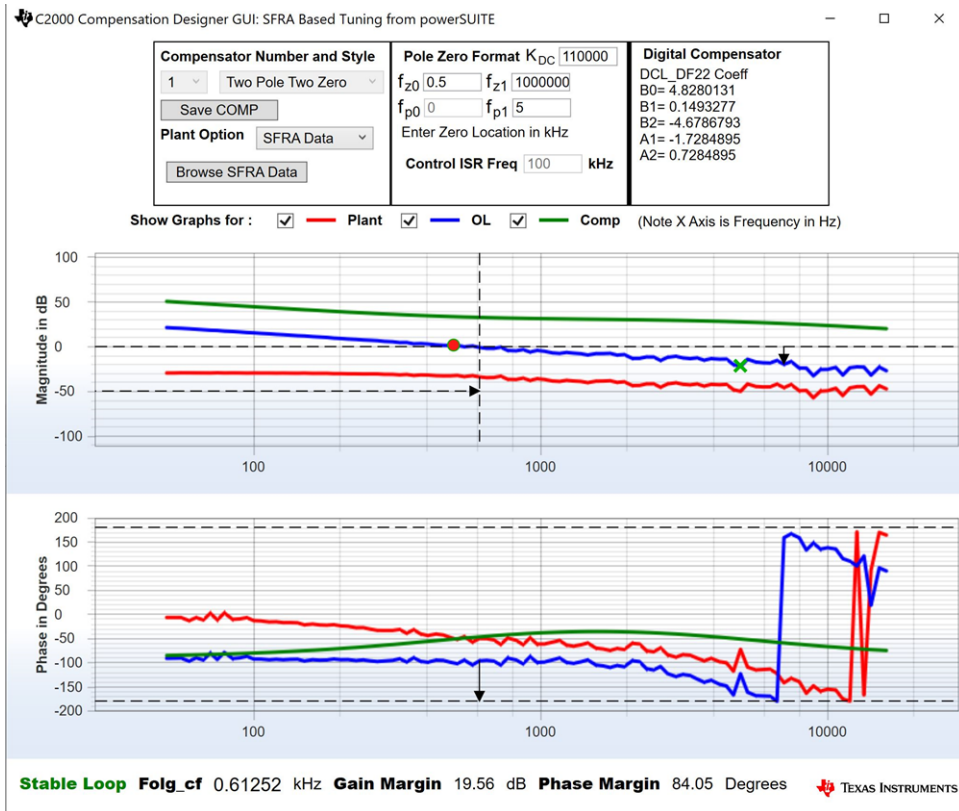
图 46. Compensator Design With SFRA Based Plant Measurement for the Voltage Loop When Resistive Load is Connected at the Output, With Measurement Data at 500kHz
