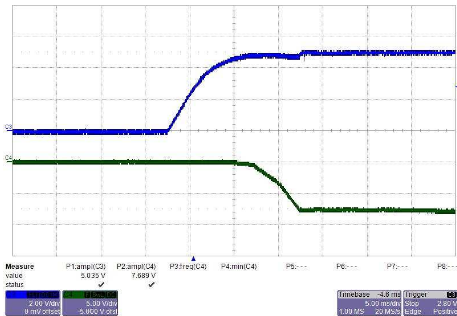
图 15. Start-up Waveform of the -9-V Rail With V_{IN} = 5\text{ V} and no Load
