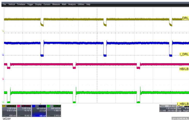
图 19. 90% PWM'ing at Low Power
