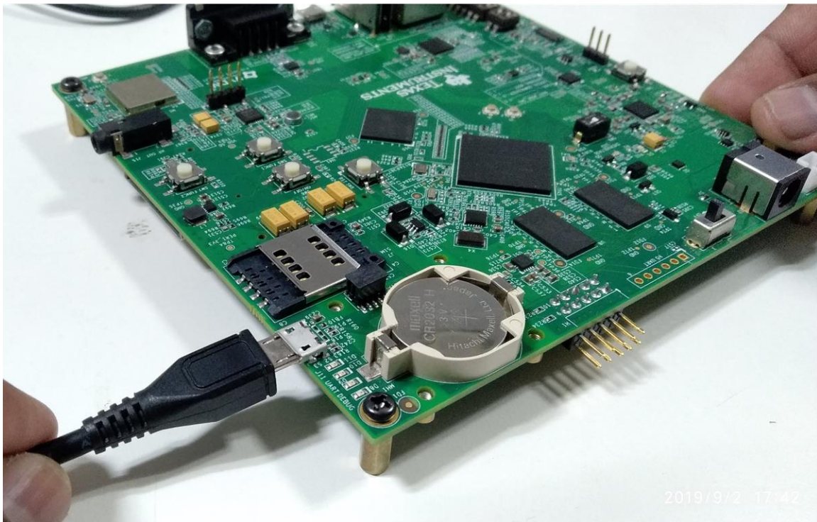
图 27. Inserting micro-B Cable Into J11
