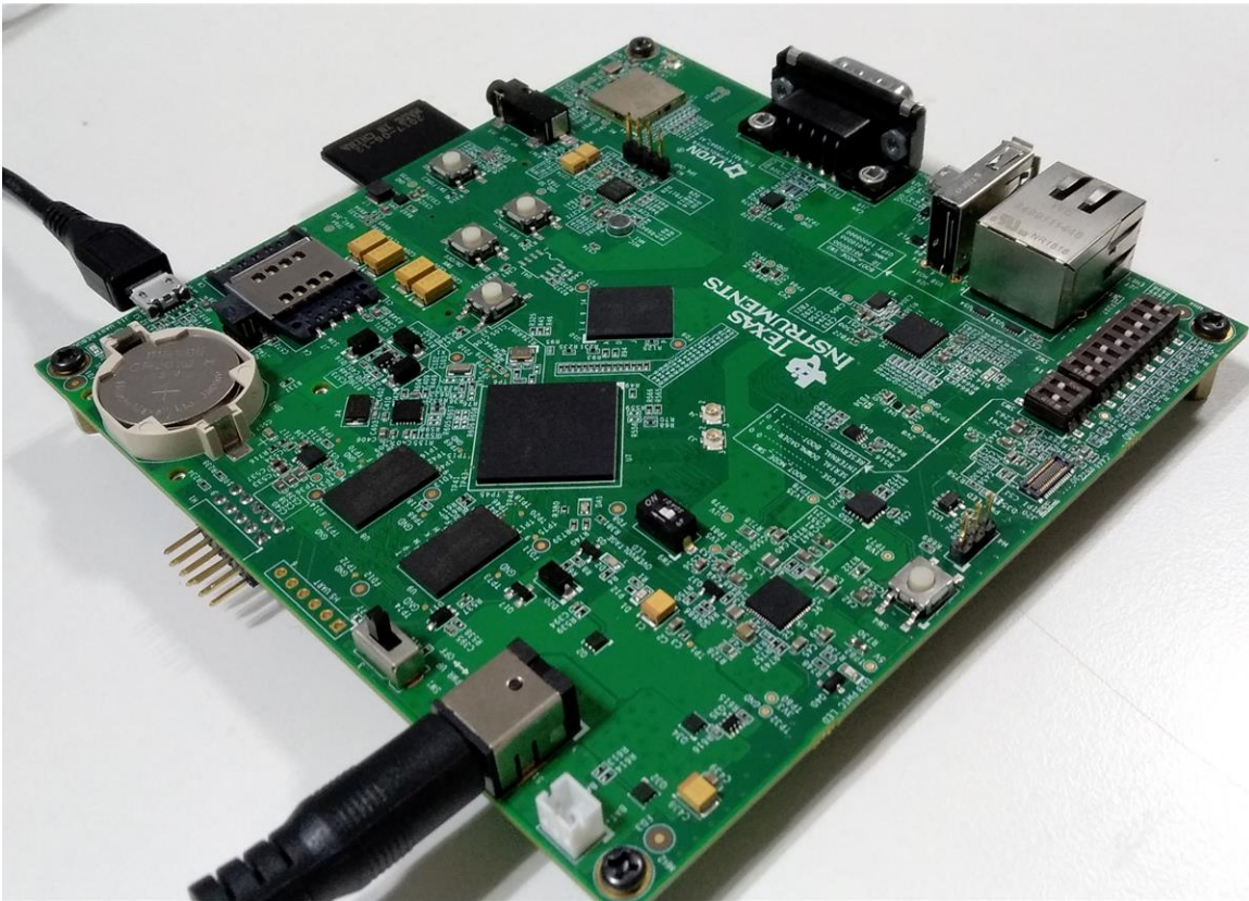
图 29. Board Connections for BOOT From SD Card With Debug Over USB
