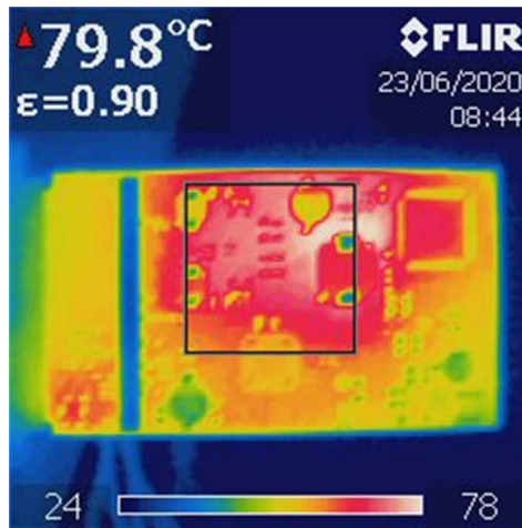
图 3-26. Bottom Side Thermal Image Highbeam/Lowbeam at 30W, Turn Indicator at 7.5W average
