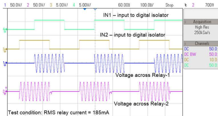
图 3-16. Test Waveforms at 24-VAC Supply - Independent Operation of SSR
