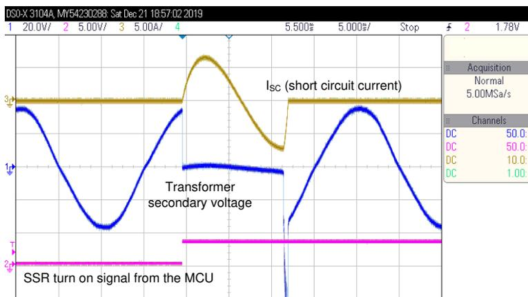
**图 3-18. Short-Circuit Test Waveforms With External Fuse**
