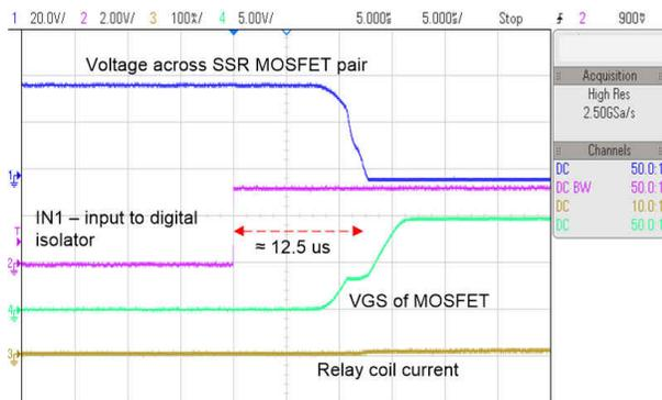
图 3-12. Waveforms Showing SSR Turn on Time
