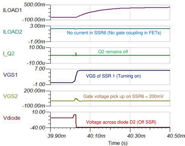
图 2-8. Simulation Results Illustrating Negligible Cross-Coupling
