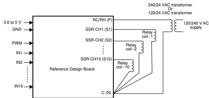
图 3-2. Interfacing External Control Signals, Relay coils and Transformer to the Board
