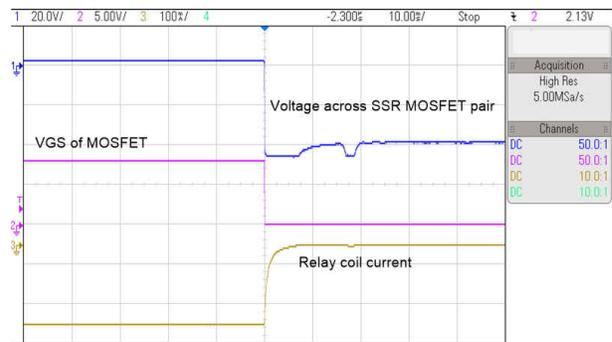
**图 3-9. SSR Turn off Waveform at -40 V**
