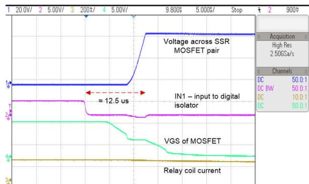
图 3-13. Waveforms Showing SSR Turn off Time
