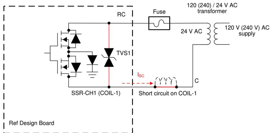
图 3-17. Overcurrent Protection Circuit With External Fuse
