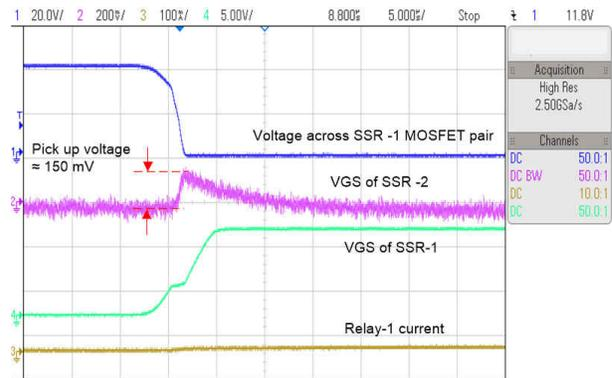
图 3-15. Test Waveforms Showing Least Cross-Coupling During SSR Turn On
