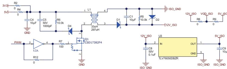
图 2-12. Open-Loop Flyback Power Supply
