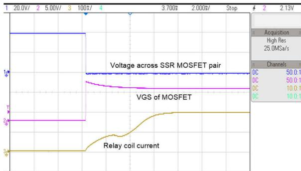
**图 3-6. SSR Turn on Waveform at 40 V**
