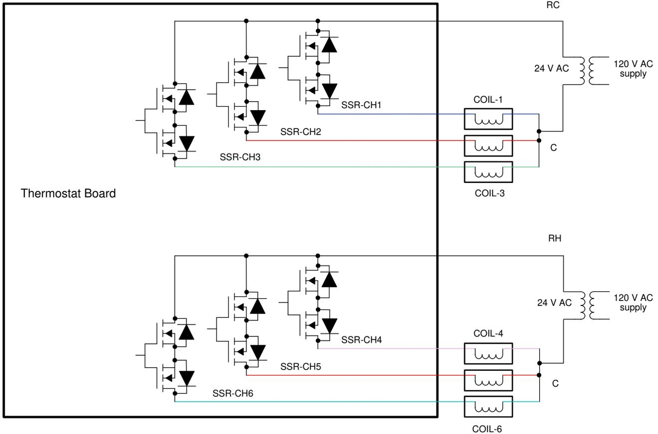
图 3-19. Circuit Topology in Driving Multiple SSRs With two AC Transformers
