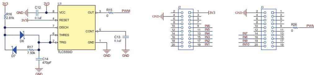
图 2-13. TIMER to Generate PWM Signal and Interface Connector
