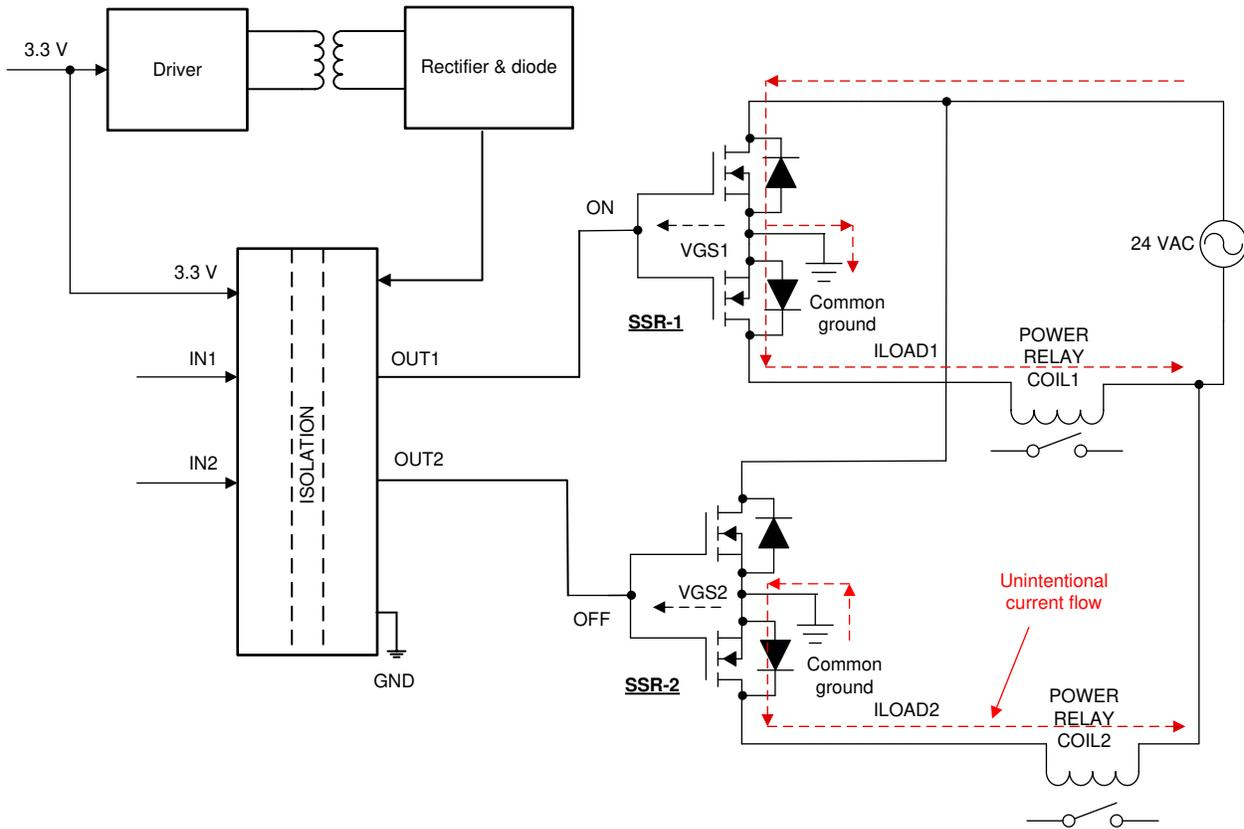
图 2-4. Unintentional Current Flow in Driving Multiple SSR With Common Ground Gate-Drive Supply
