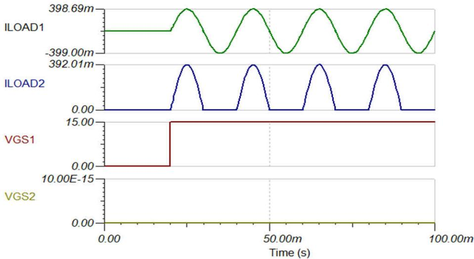
图 2-5. Half-Wave Rectified Current in Driving Multiple SSR With Common Ground Gate-Drive Supply
