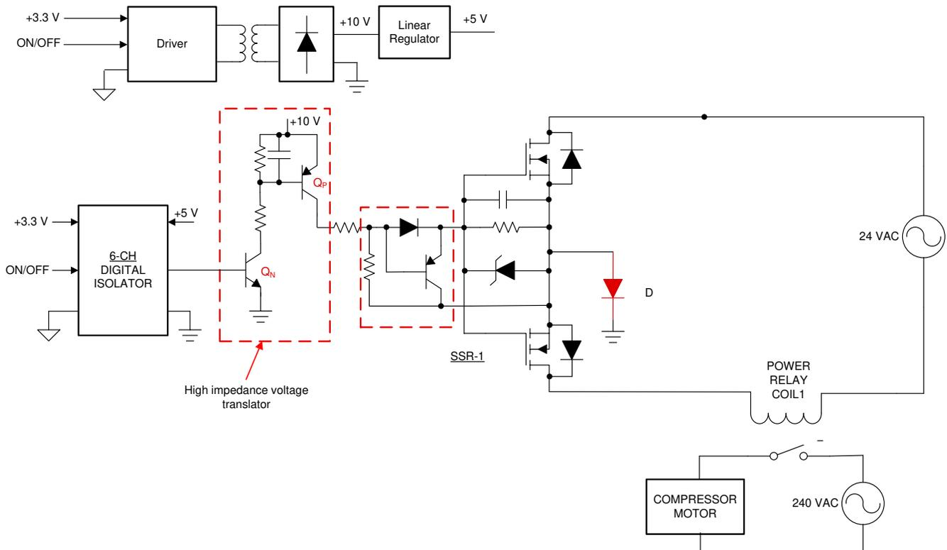
图 2-7. High Impedance Voltage Translator for Driving Multiple SSR With Single Isolating Element
