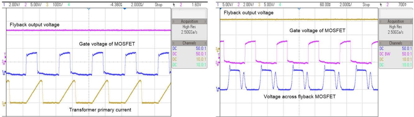
**图 3-5. Flyback Circuit Voltage and Current Waveforms - All SSR Off**
