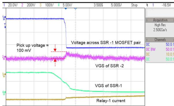
图 3-14. Test Waveforms Showing Least Cross-Coupling During SSR Turn Off
