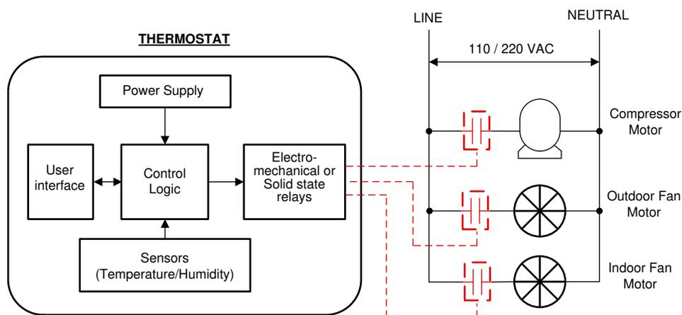
图 2-1. Multiple Relays Controlling Different Loads in Thermostats
