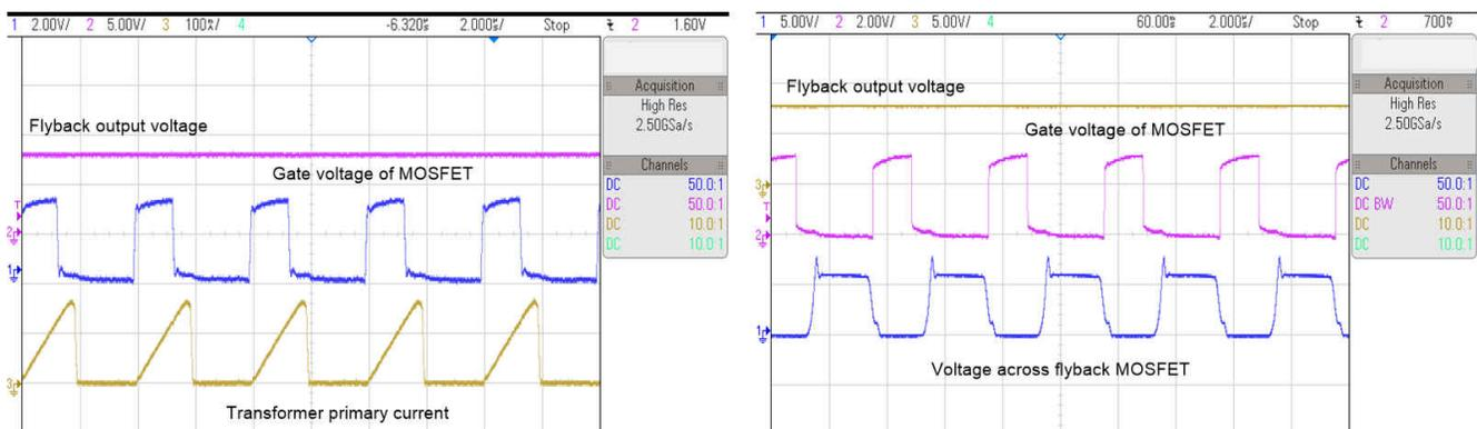
图 3-4. Flyback Circuit Voltage and Current Waveforms - All SSR On
