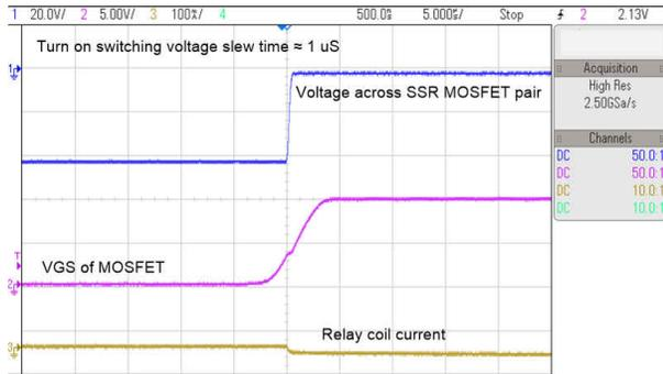
图 3-10. MOSFET Turn on Switching Waveform
