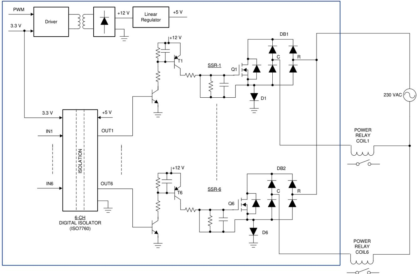
图 3-20. Circuit Topology for Cost Reduction at High Voltage
