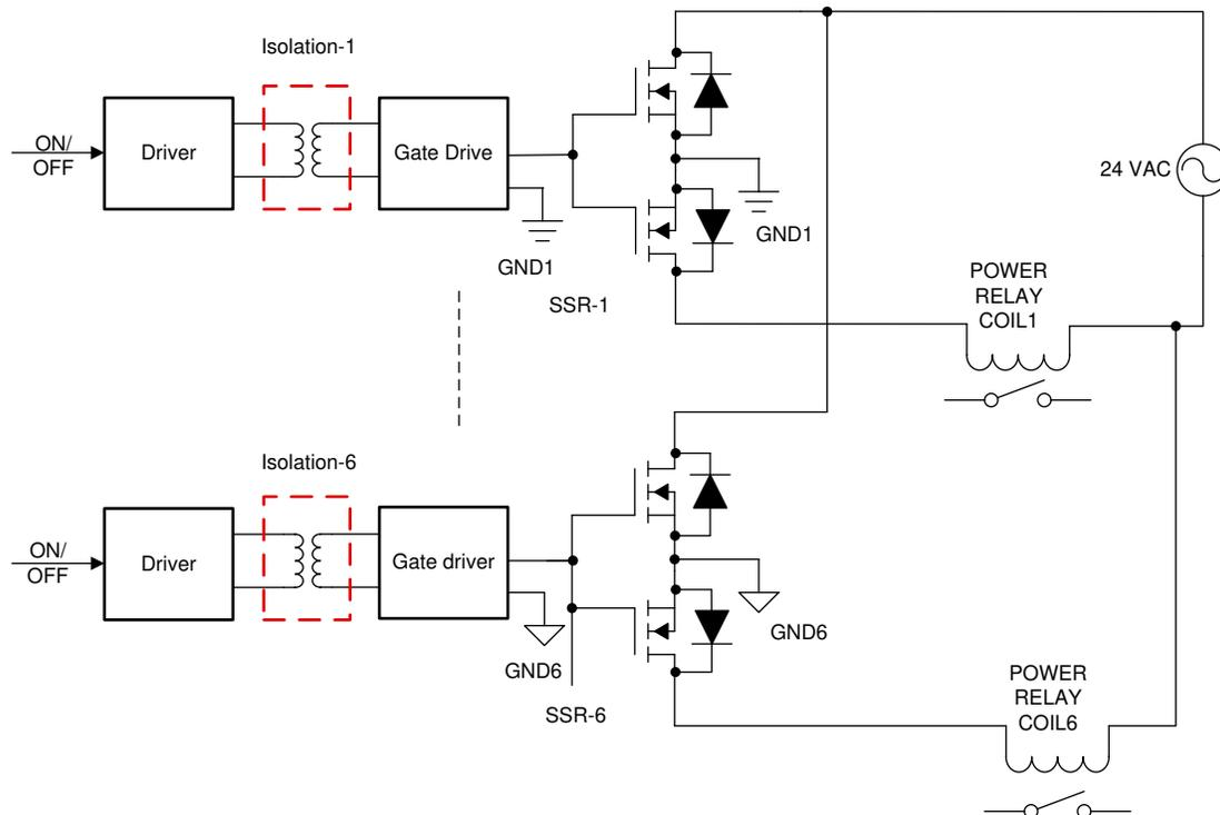
图 2-3. Multichannel SSR Topology With Independent Isolation Between SSR Channels
