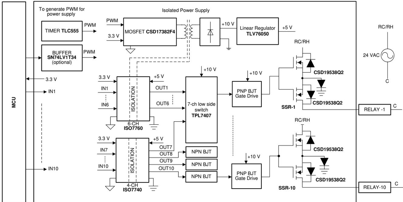
图 2-2. TIDA-010085 Reference Design Block Diagram
