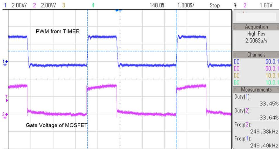
图 3-3. PWM Signal from the MCU or TIMER and MOSFET Gate-Source Voltage
