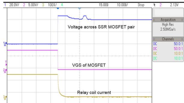
**图 3-7. SSR Turn off Waveform at 40 V**
