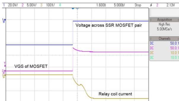
**图 3-8. SSR Turn on Waveform at -40 V**
