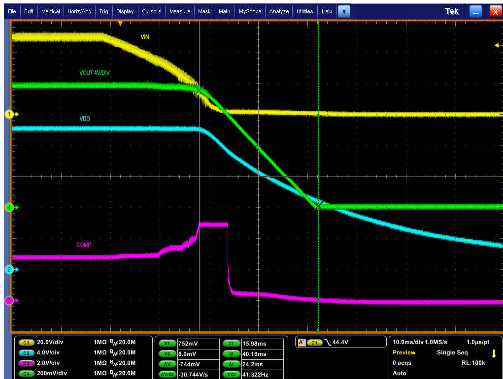
图 5-12. 关断，VIN 移除：VIN = 50V，负载 = 1.3A
