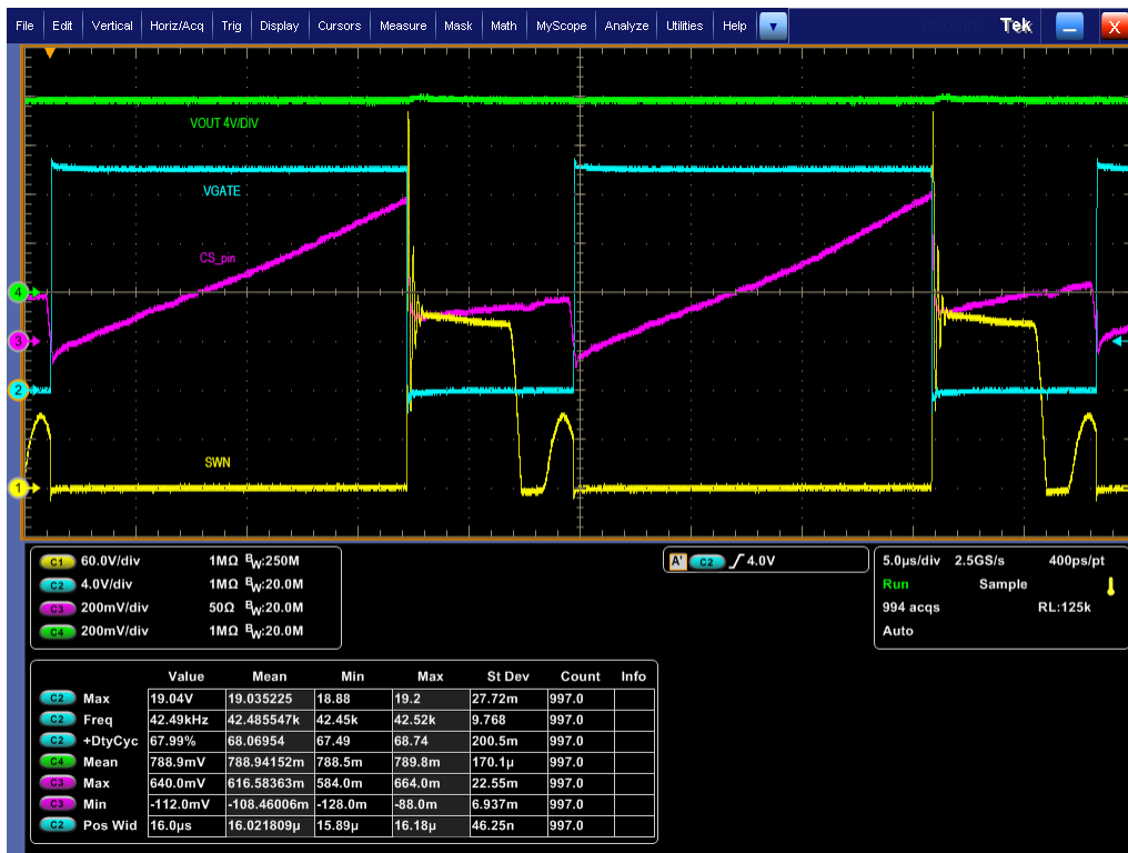
图 5-20. 稳态 : V_{IN} = 50V , 负载 = 1.3A
