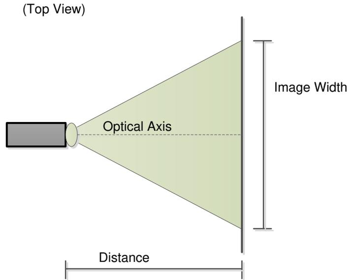
$$\text{Throw Ratio} = \text{Distance} / \text{Image Width}$$
