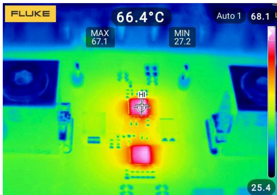
图 5-18. TPS25990EVM 的热性能 ( V IN = 12V , R IMON = 0.91 // 1.1kΩ , V IREF = 1.13V , I OUT = 110A )
