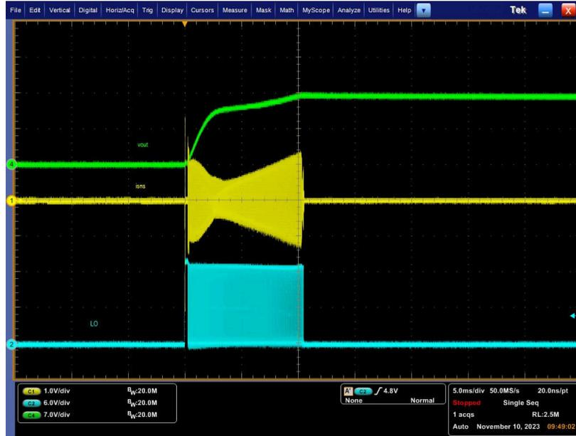
图 3-1. 无负载 (0A) 启动 ( Ch1 = ISNS ; Ch2 = LO ; Ch4 = V<sub>OUT</sub> )
