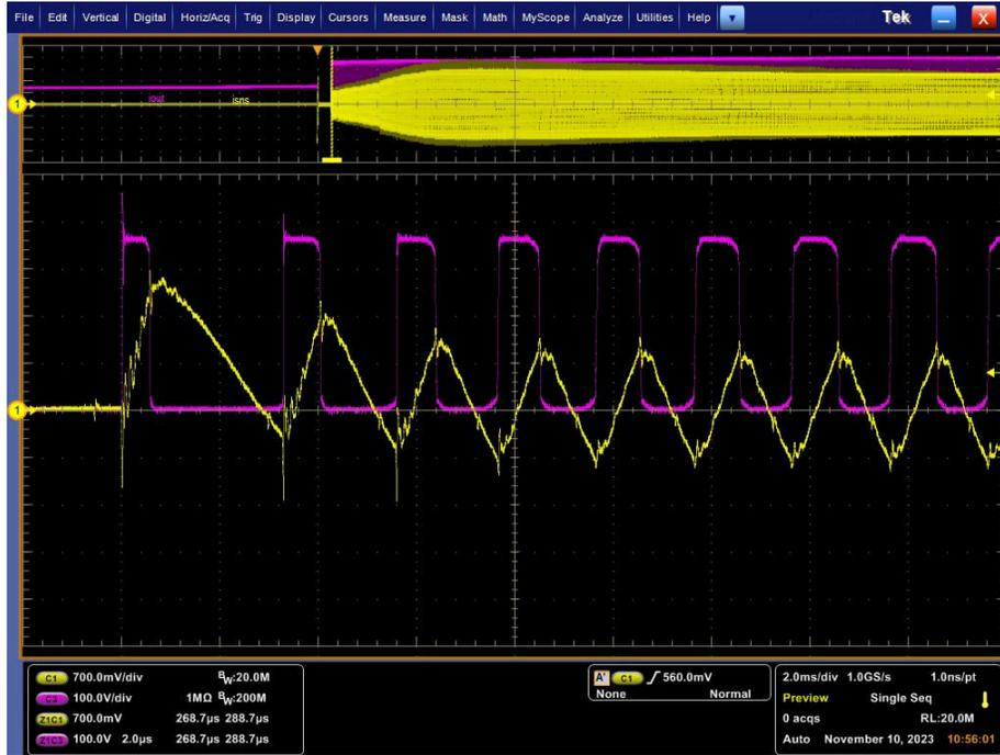
图 3-3. 满载 (15A) 启动 ( Ch1 = ISNS ; Ch3 = SW )
