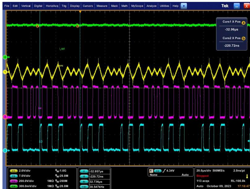
图 3-11. 1A 负载时的稳态波形 ( Ch1= ISNS ; Ch2 = LO ; Ch3 = SW ; Ch4 = I\_OPT )
