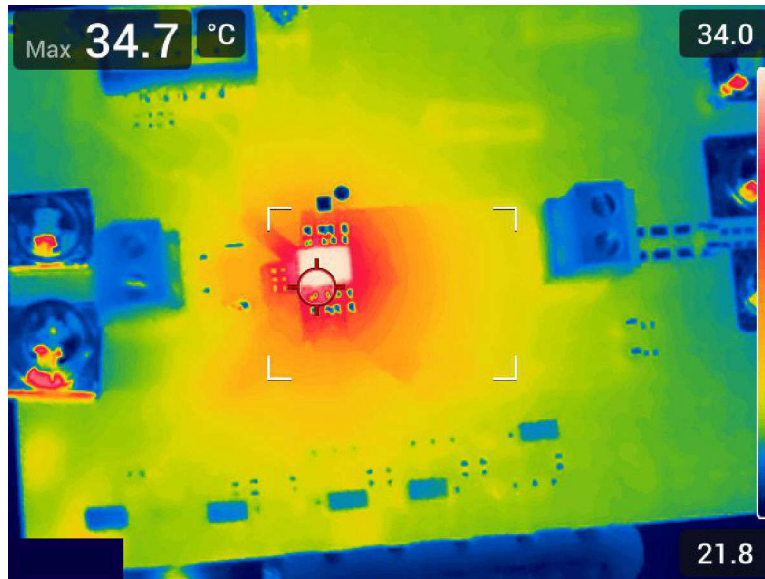
图 4-3. 热性能 (TPSM8287A10BAHEVM, V_{IN} = 5V , V_{OUT} = 0.9V , I_{OUT} = 10A )
