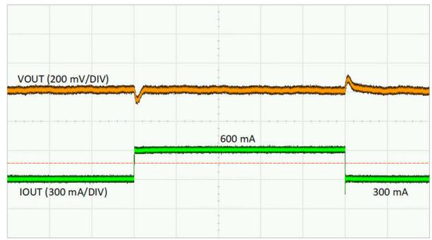
图 3-8. 负载瞬态,  $12V_{IN}$ ,  $3.3V_{OUT}$ ,  $I_{OUT} = 300mA$  至  $600mA$ , 压摆率 =  $1A/\mu s$  (自动)
