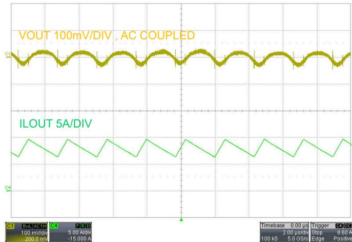
图 3-5. 输出纹波,  $V_{\text{SUPPLY}} = 48\text{V}$ ,  $I_{\text{LOAD}} = 8\text{A}$
