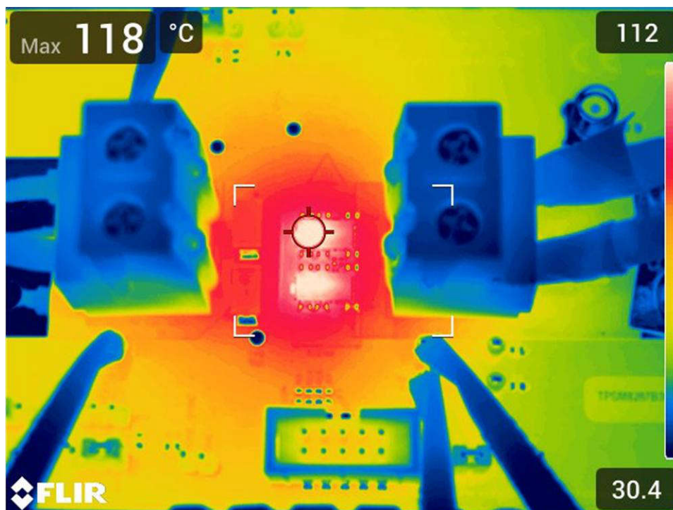
图 4-1. 热性能 (TPSM8287B30-2X-EVM, V_{IN} = 5V , V_{OUT} = 0.6V , I_{OUT} = 60A )
