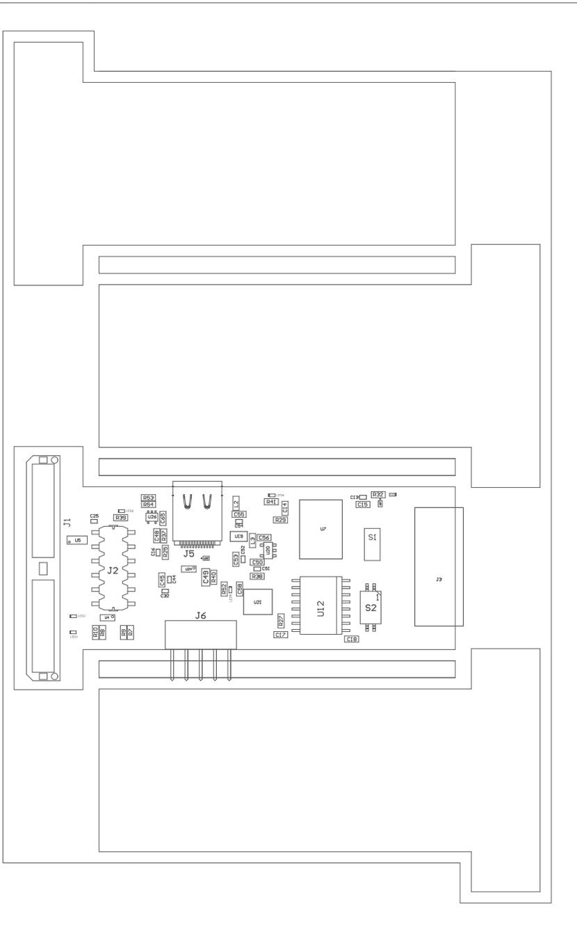
Z24 ■ These assemblies must comply with workmanship standards IPC-A-610 Class 2, unless otherwise specified.
